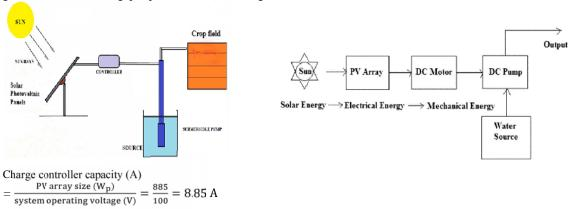
**Fig. 1.** Layout of solar PV water pumping system.
